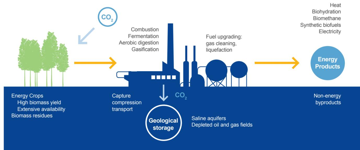
CCU is a simple concept: Gas and particle waste produced from industrial sources like power plants, steel making or other factories is first captured. The carbon from that waste is then extracted using chemical processes and reused as the raw material for new products. Reusing this carbon not only decreases CO<sub>2</sub> emissions into the atmosphere, but also decreases fossil fuel use.
