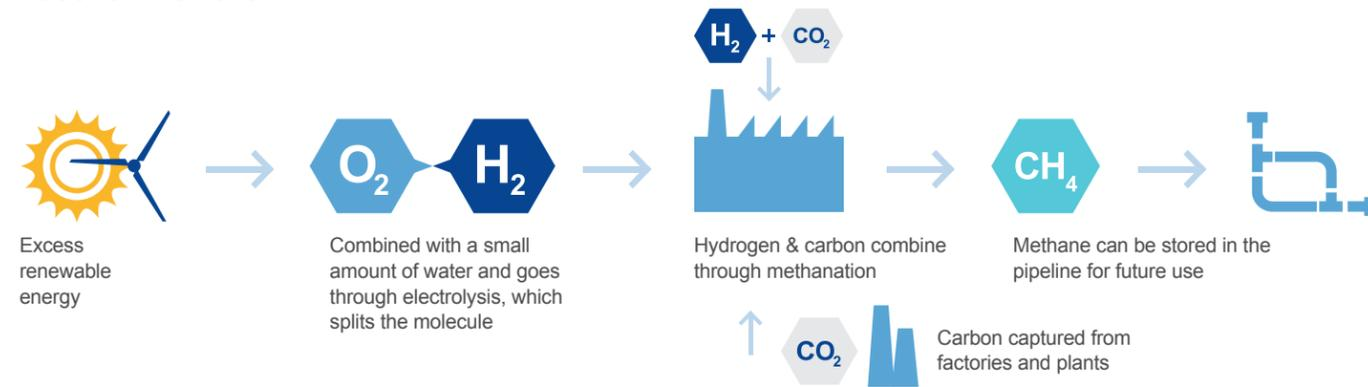
Power-to-Gas works by taking excess electricity generated from solar and wind, combining it with a small amount of water and running it through electrolysis. The electrolysis process converts the electrical energy into chemical energy and splits the molecules into pure hydrogen and oxygen.
