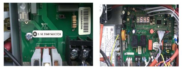
The Robur unit is operated by a microprocessor control. The diagnostic control registers supply and return water temperatures and allows for ease of service and faster trouble shooting if necessary.
