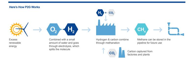
Power-to-Gas works by taking excess electricity generated from solar and wind, combining it with a small amount of water and running it through electrolysis. The electrolysis process converts the electrical energy into chemical energy and splits the molecules into pure hydrogen and oxygen.
