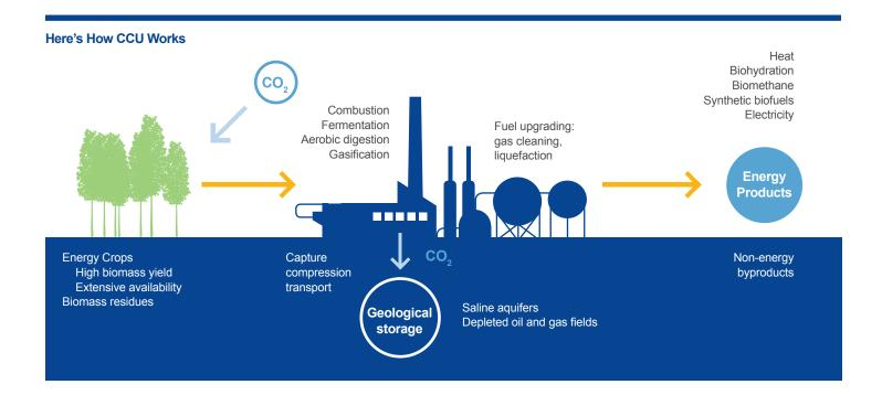
CCU is a simple concept: Gas and particle waste produced from industrial sources like power plants, steel making or other factories is first captured. The carbon from that waste is then extracted using chemical processes and reused as the raw material for new products. Reusing this carbon not only decreases  $\mathrm{CO}_2$  emissions into the atmosphere, but also decreases fossil fuel use.
